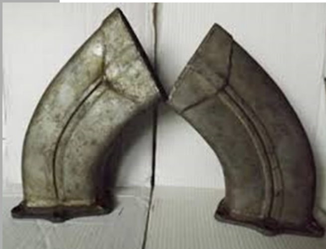
Confirmed, the stubs to our Merlin matched those on Lancasters
